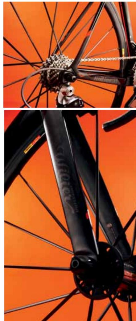
to extend the depth of the head tube and consequently improve stiffness and handling without creating a tall overall head tube height. 'They call it a virtual head tube as all this extra carbon stiffens the head tube up,' Izzard says.
